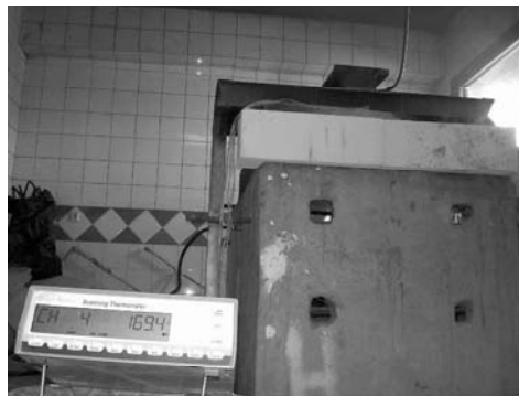
Fig. 11. Fire chamber for slabs.
