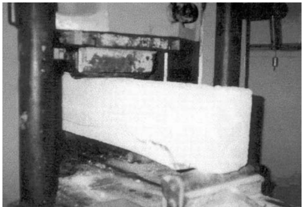
Plate 1. Peeling failure mode for the beam strengthened in tension at bottom.
