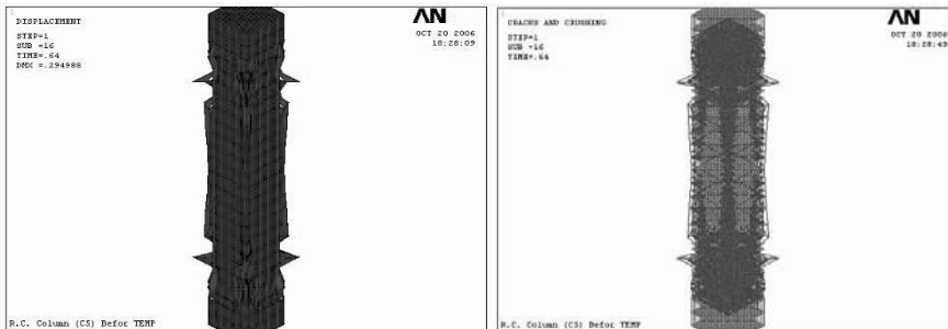
Fig. 4d. Deformed shape and first crack of column no. C5 15 min. after fire.
