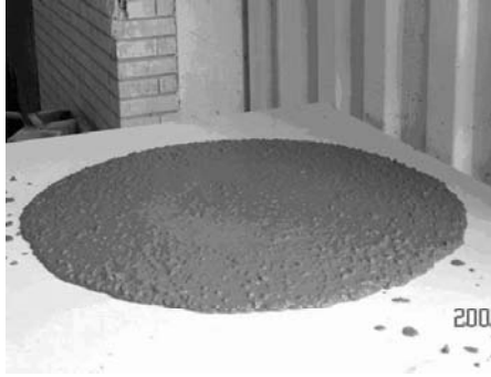
Fig. 1. Slump flow test.
