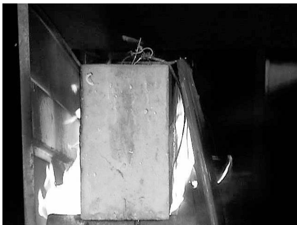
Fig. 5. Fire testing of a beam specimen.
