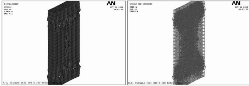
Fig. 4b. Deformed shape and first crack for column no C2 before exposure to fire.
