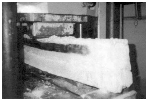
Plate 2. Failure mode for the beam strengthened in compression at side.
