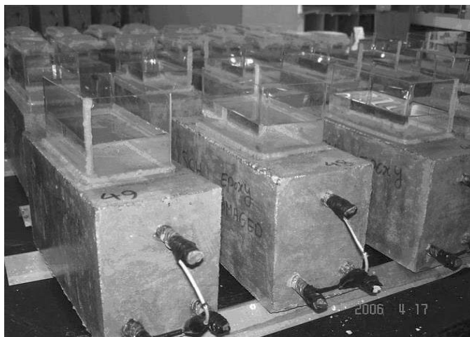
Fig. 5: Concrete specimens according to ASTM G 109-92
