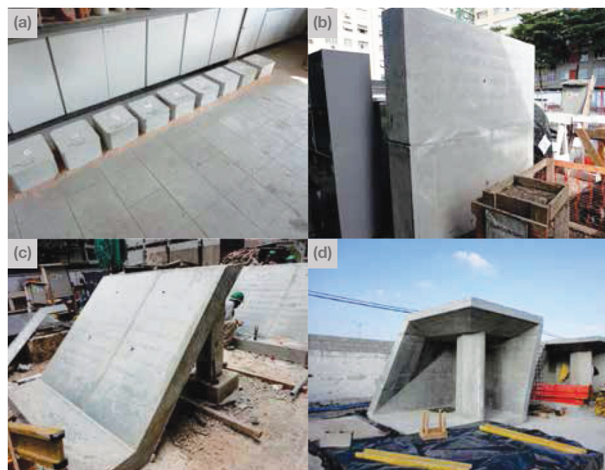
Fig. 3: Various simulations and mockups used to establish materials and methods incorporated in the building construction: (a) cubic specimens in the laboratory of the concrete supplier, October 2011; (b) vertical wall cast at the jobsite, February 2012; (c) inclined wall (45 degrees) cast at the jobsite, February 2012; and (d) full-scale mockup cast in the courtyard of the concrete supplier's plant, July 2012
