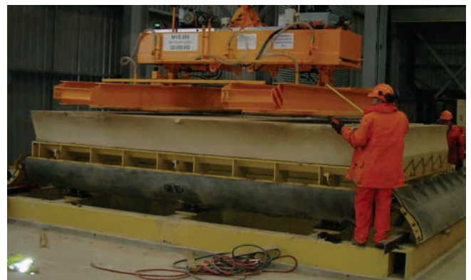
Revetment unit being vacuum-lifted out of the mould
