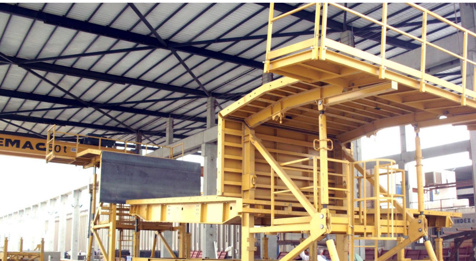
Molds being assembled in production line
