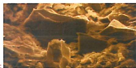
Fig d: Microscopic examination reveals the Glassy nature of GGBS particles
