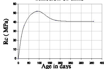
Fig.5 Compressive strength as function of time
