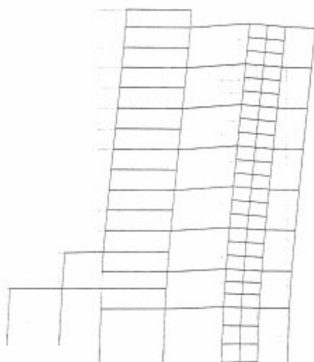
Figure 3b. Second mode of a typical frame.
